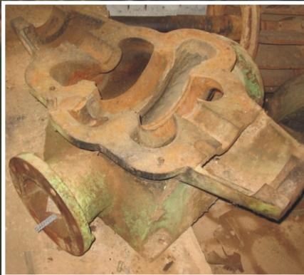
This Brazilian paper mill stock pump was severely damaged after 12 years of continuous use. The mill's engineers sent the pump out to two separate pump repair companies who advised that this pump was "unrepairable" and suggested replacement as the only viable option.
