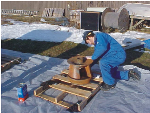
Impellers placed on pallets outdoors and then grit blasted to minimum 3 mil profile.
