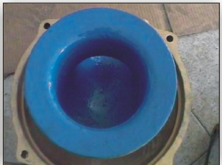
DuraTough DL applied to completely seal and protect the discharger.
