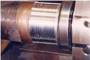
The shaft of this vessel's hydraulic anchor winch was found badly in need of repair during a routine maintenance inspection in Israel.
