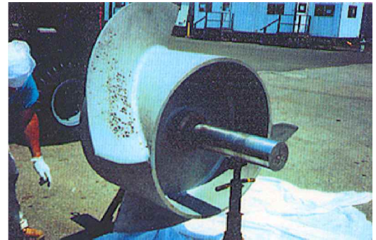
The pump impeller, after grit blasting.
